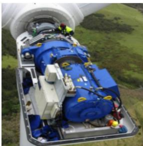
Figure 1.8 Example of the drivetrain of a wind turbine [19]
