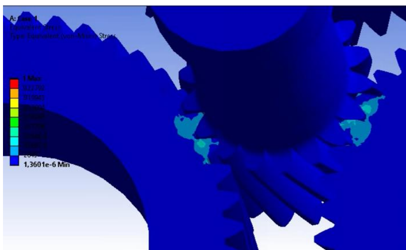
Figure 4.14 Results of SF in the case study of the shaft rotates at 8.88 rpm and there is no wind effect from the blade to the shaft
